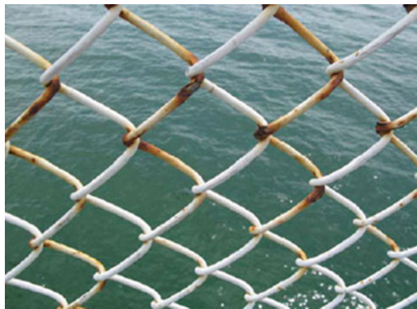
Fig. 13.48 Higher stress regions (and more plastic deformation) occur at the crossover bending points of this chain-link fence. Note the enhanced corrosion rates at these crossover/bent-wire locations. Also note that for each bend, the top surface (in tension) generally shows more corrosion than does the underneath surface (in compression)
