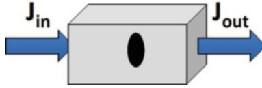
Fig. 5.1 Material degradation (voiding or accumulation of material is shown in darker region of volume V of interest) occurs due to a flux divergence. J_{in} represents the flux of particles into the volume V of interest and J_{out} represents the flux of particles out. The volume V of interest is bounded by a surface of area A . Flux divergence occurs if J_{in} \neq J_{out}
